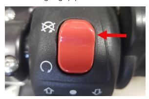
Note that when this switch is in the Off position, the motors are off, but all electronic functions are available (see page 5). Switch the Emergency Off switch to the OFF position.
