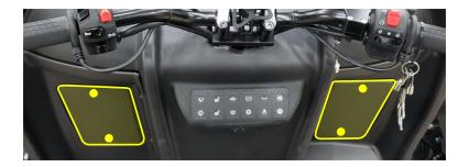
With these panels removed, you have access to the left and right side service ports.
