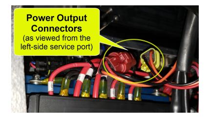
Press the locking tab down, and gently pull to unplug each connector.
