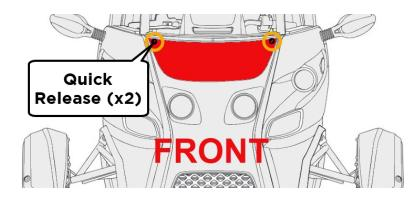
Twist both Quick Release thumbscrews counter-clockwise to release the panel.
