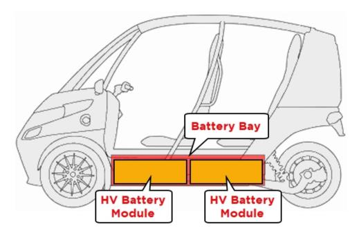
Each Battery Module is enclosed in a sealed case and bolted to the floor of the Battery Bay. These Battery Module are designed to be water and impact resistant.
