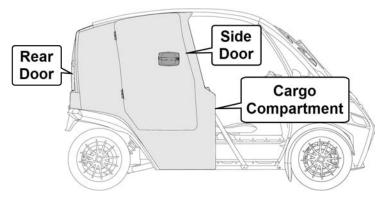
The Cargo Compartment includes a hinged shelf and vinyl cargo divider to help organize and secure the load.
