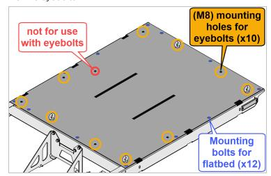
Eyebolts (four included) can be installed in any of these mounting locations. Note that there is one hole in the flatbed cargo carrier that should NOT be used with eyebolts, as indicated above
