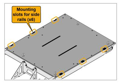
Secure each side rail with two M8-1.25 mounting bolts.Torque bolts to 8 Ft-LBS.
