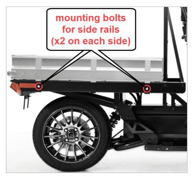
3. Slide each side rail straight up and out of the mounting holes on the flatbed.
